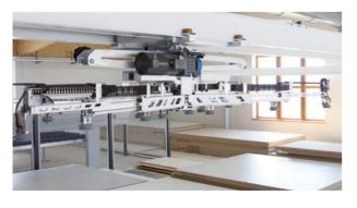
The highlight of the STORETEQ S-200 is its combination with suction traverse ST 71.
